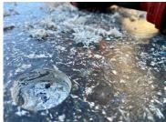
**Colouring** of the edge can be made by colouring the epoxy to achieve a matching or contrast colour to the facing. For small applications the use of food colouring is an option to colour the epoxy.
