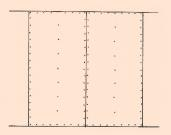
Sheet layout - All edges must be supported - Sheets to be installed vertically
