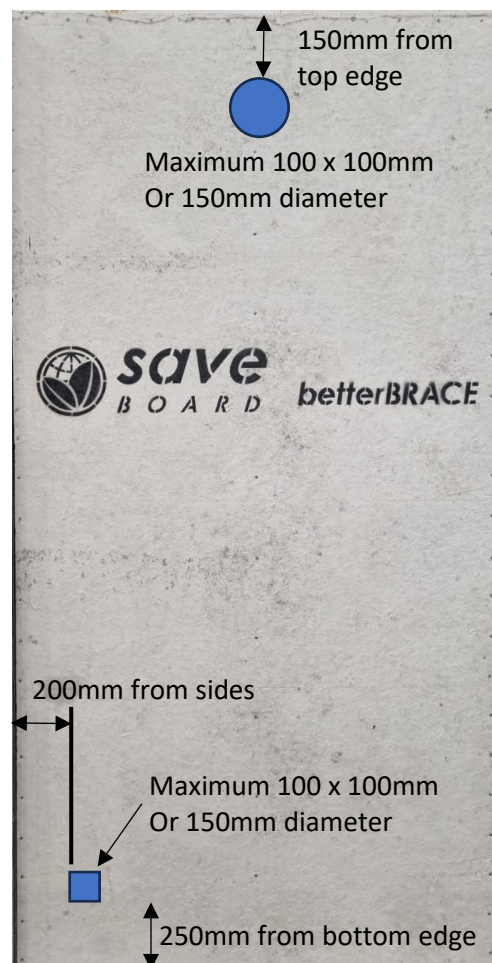
DIAGRAM 8 – Permitted penetrations in Bracing board. Note: All penetrations are to be sealed as per the instructions in this guide.
