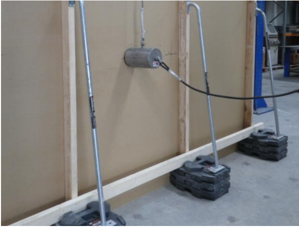
FIG. 4 IMPACT TEST SETUP
