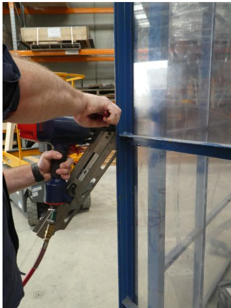
FIG. 2 NAIL PENETRATION TEST SETUP
