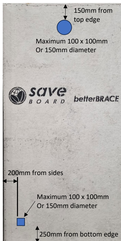
DIAGRAM 8 – Permitted penetrations in Bracing board. Note: All penetrations are to be sealed as per the instructions in this guide.
