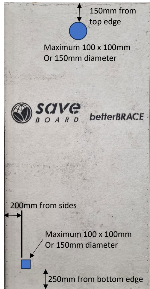
DIAGRAM 6 – Permitted penetrations in Bracing board. Note: All penetrations are to be sealed as per the instructions in this guide.
